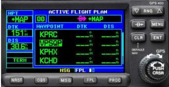
To enter +MAP into your flight plan, activate the cursor (press the small button labeled PUSH CRSR).
