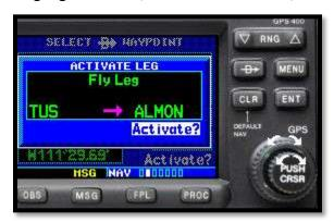
Press DCT DCT and ENT
